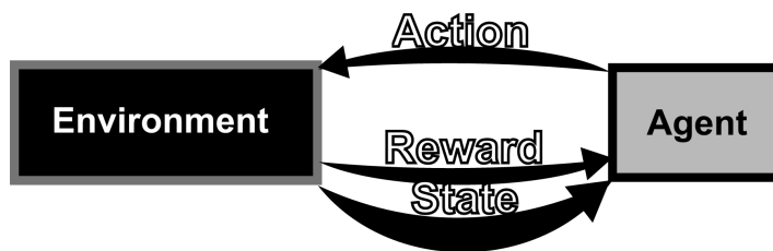
FIGURE 1.1: The Agent Environment Loop: the cycle of the agent taking actions and the environment telling the agent how the state changed and how good the action was (reward value).
